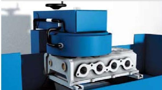
3. Remove any gouging, component distortions, grooves or scores, e.g. by surface grinding in a specialist workshop.
