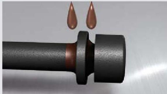
10. If the manufacturer specifies the use of a washer, lightly lubricate both sides.
