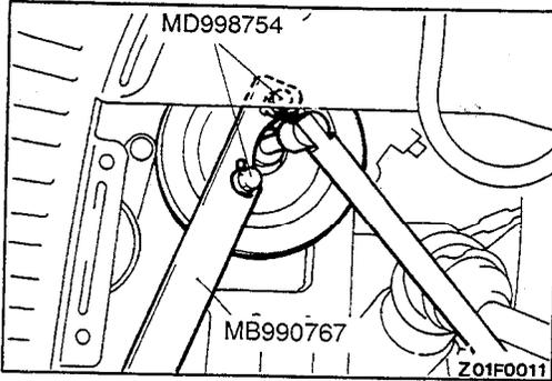
**REMOVAL SERVICE POINTS****◀A▶ CRANKSHAFT PULLEY REMOVAL**
